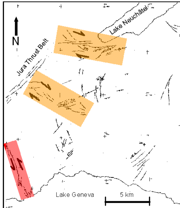
Figure 10: Sketch map of faults in the Top Dogger sequence from seismic data between Lake Neuchâtel and Lake Geneva. Three major strike-slip fault systems are highlighted.
